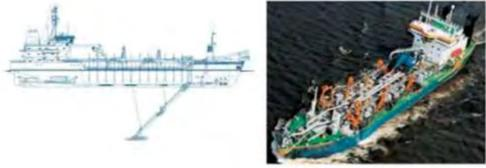
Gambar 2.7 Trailing Suction Hopper Dredger (TSHD) (Sumber: Pullar, 2009)
