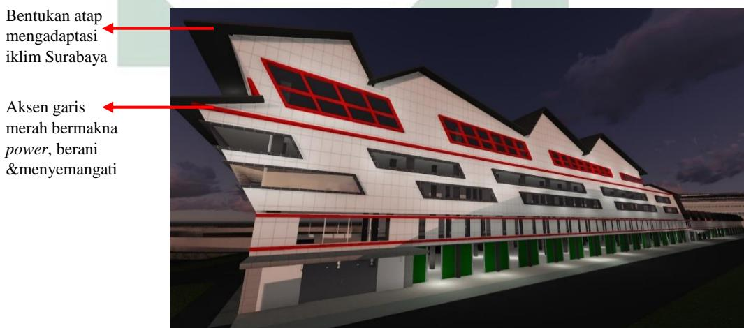
Gambar 4.3 *Pit Building* bagian focal point
