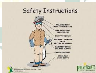
Picture 4.6 Safety Welding Equipment
