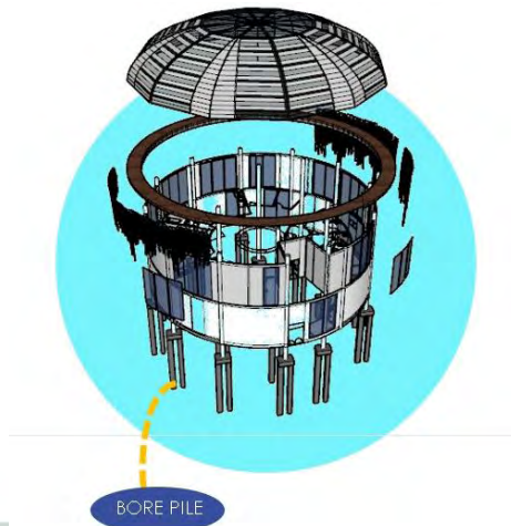
Gambar 4. 10 Pondasi Bore Pile
