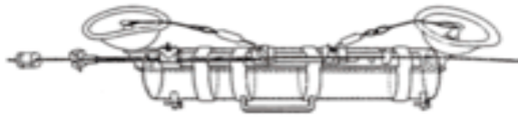
Gambar 2. 2 Water Sampler Sumber Gambar : SNI 6989.57.2008
