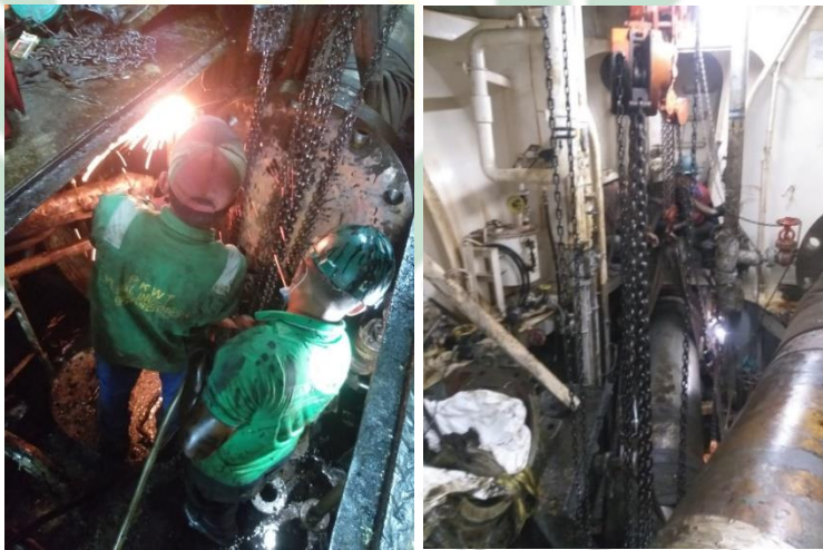
Gambar 3.4 Perbaikan as propeller
