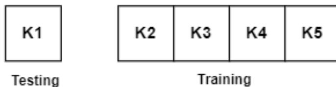
Gambar 3. 3 Skenario *K-fold Cross Validation*
