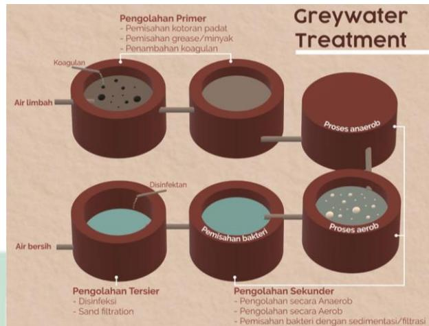
Gambar 4.32 Tahapan pengolahan air greywater
