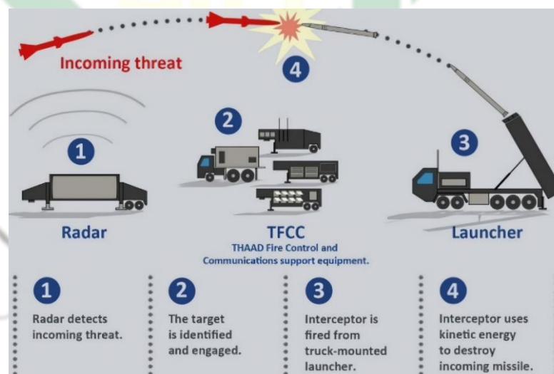
Gambar 2.1 Sistem Kerja Terminal High Altitude Area Defense. Sumber: THAAD in the Korean Peninsula . 2016. Institute for Security and Development Policy. https://isdps.org/publication/korea-thaad/
